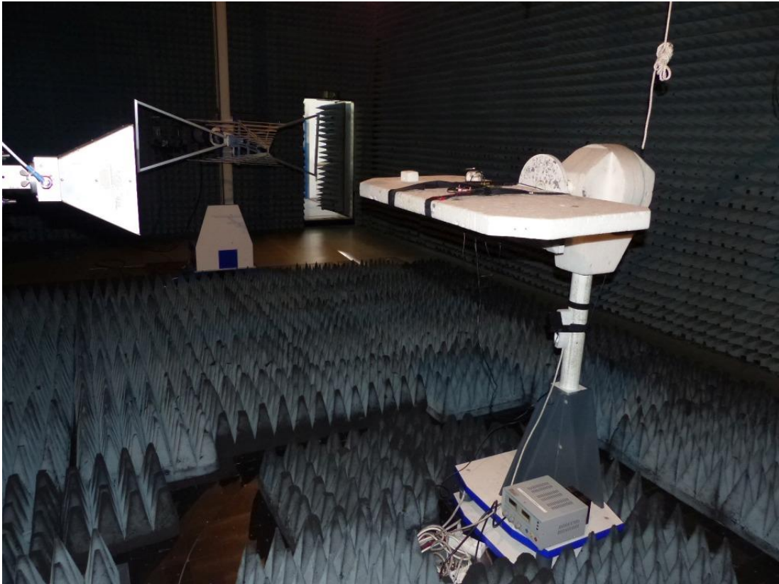
Photo 5: Test setup for radiated measurements (Enclosure, fully-anechoic chamber, 1-18 GHz intentional radiator §15 / 30 MHz – 10/20 GHz §22/24/27)
