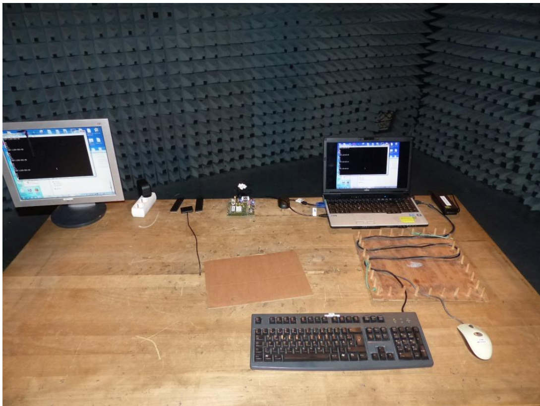
Photo 1: Test setup AA01 for radiated measurements unintentional radiator §15) Single device setup, computer peripheral.
