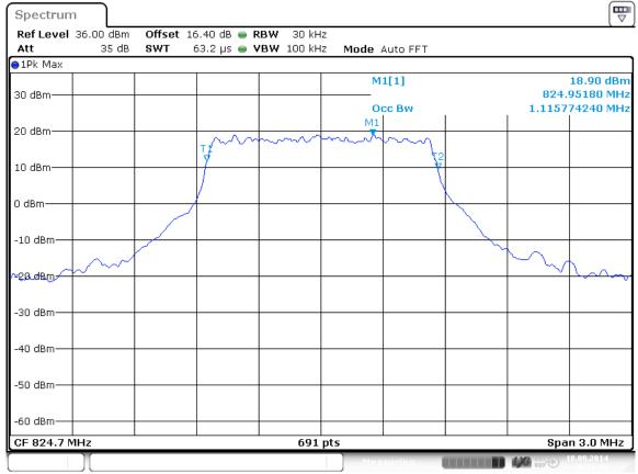
Channel 20407, CBW 1.4MHz, RB/Offset 6/0, Modulation QPSK
