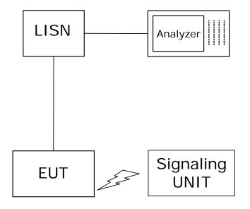
Setup in the shielded room for conducted measurements at AC mains port
