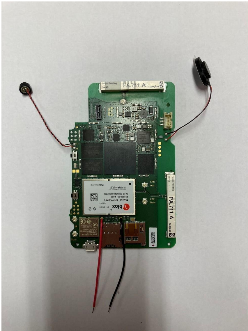
Front side Main PCB with EMC shield cans Removed
