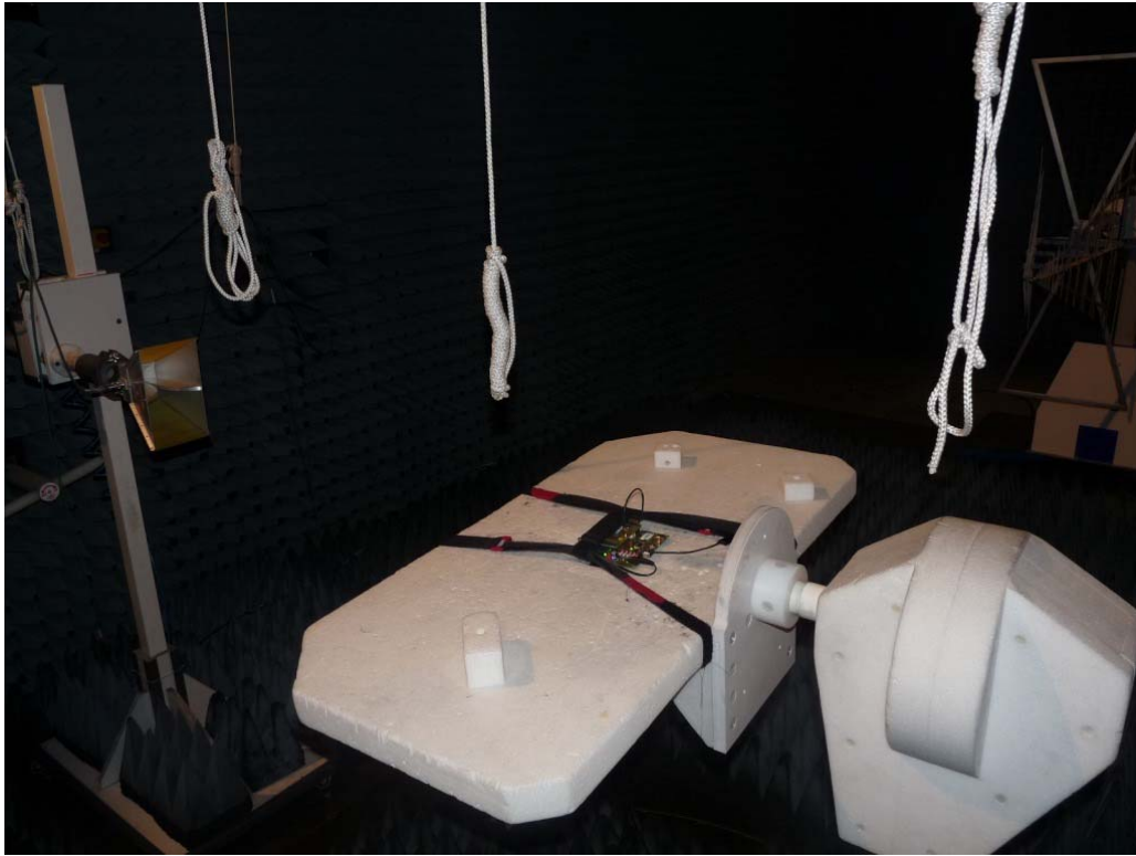
Photo 1: Test setup for radiated measurements (Enclosure, fully-anechoic chamber, §15 / 30 MHz – 10/20 GHz §22/24/27)
