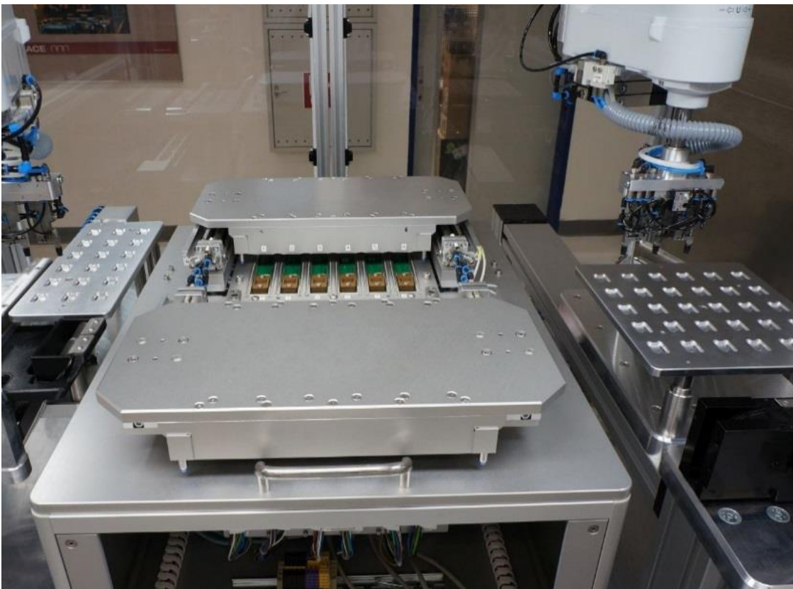
Figure 15: Automatic test equipment for module test
