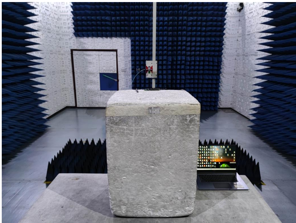
RADIATED EMISSION TEST SETUP ABOVE 1GHz
