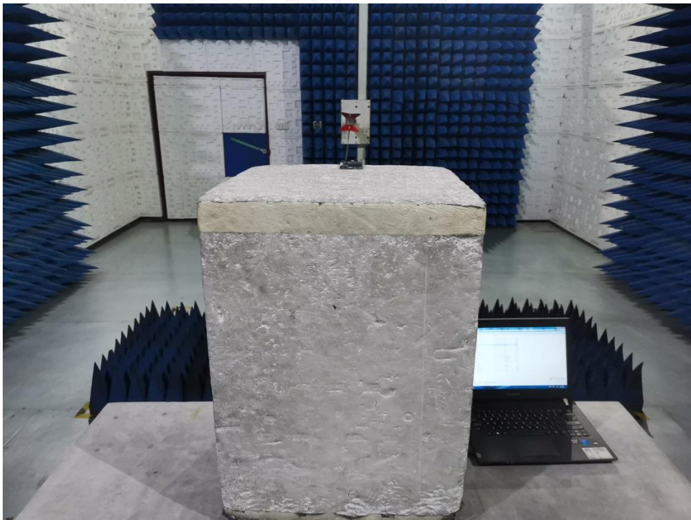
RADIATED EMISSION TEST SETUP ABOVE 1GHZ-NORA-B106
