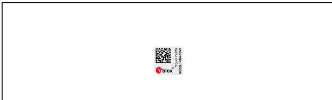
Figure 2: Actual size of the NORA-B100, NORA-B101, NORA-B106 identifier marking (8 x 8 mm)
