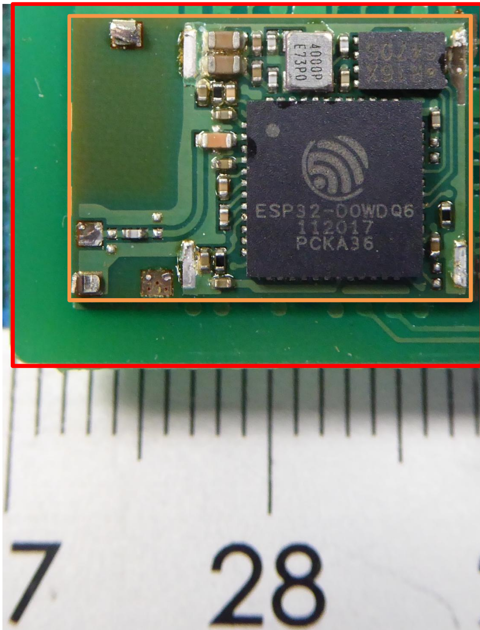
170297_E8_21.jpg: EUT (with onboard antenna removed) without shielding on not marketed eval board
