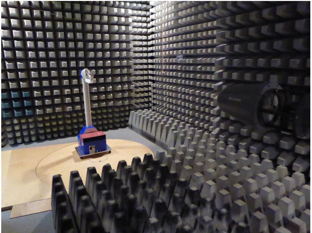
170297_E6_05.jpg: Test setup fully anechoic chamber
