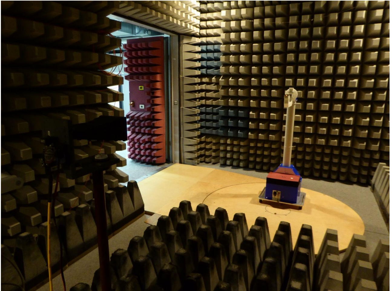
170297_E6_06.jpg: Test setup fully anechoic chamber
