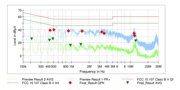
Data record name: AC powerline conducted FCC WLAN.rtf
