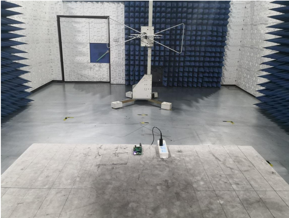
RADIATED EMISSION TEST SETUP ABOVE 1GHZ
