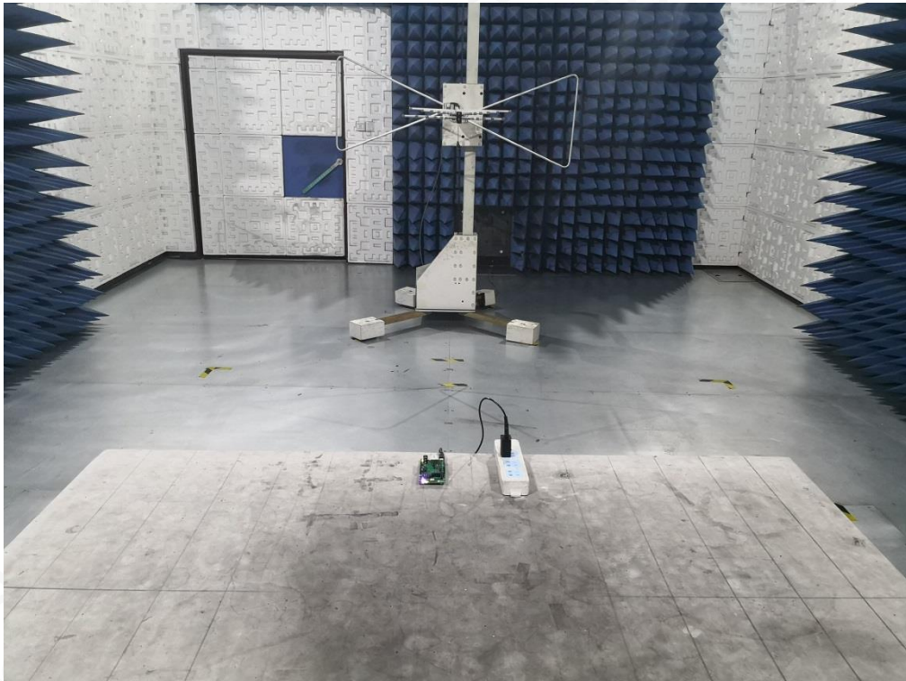
FCC RADIATED EMISSION TEST SETUP ABOVE 1GHZ
