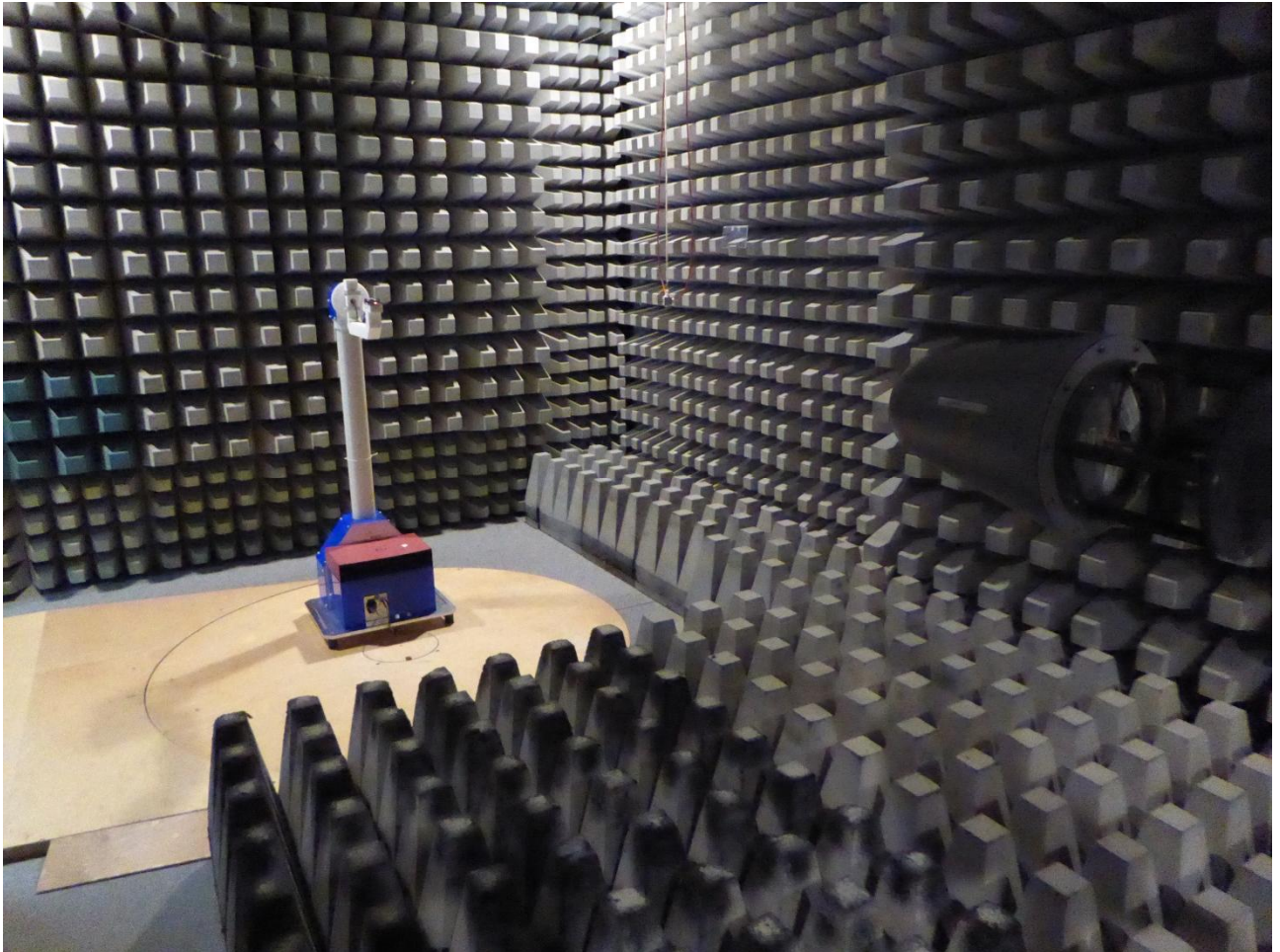
170297_E6_05.jpg: Test setup fully anechoic chamber
