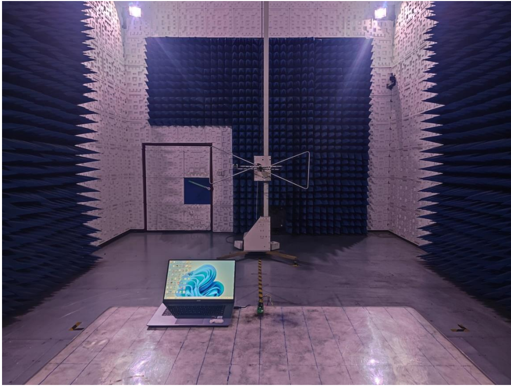
RADIATED EMISSION TEST SETUP ABOVE 1GHZ
