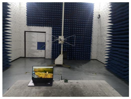
RADIATED EMISSION TEST SETUP ABOVE 1GHZ
