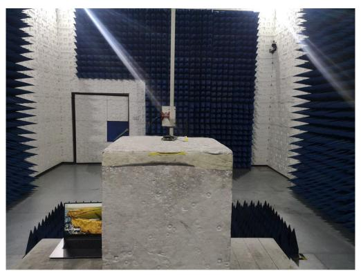
NINA-B411 of antenna 3 RADIATED EMISSION TEST SETUP BELOW 1GHZ
