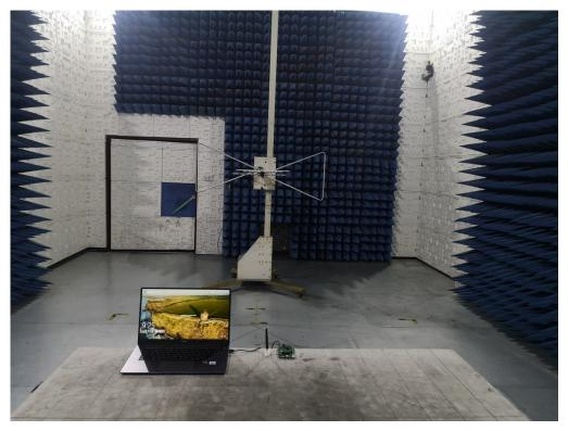
RADIATED EMISSION TEST SETUP ABOVE 1GHZ
