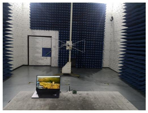
RADIATED EMISSION TEST SETUP ABOVE 1GHZ
