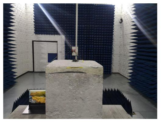
NINA-B401 of antenna 3 RADIATED EMISSION TEST SETUP BELOW 1GHZ
