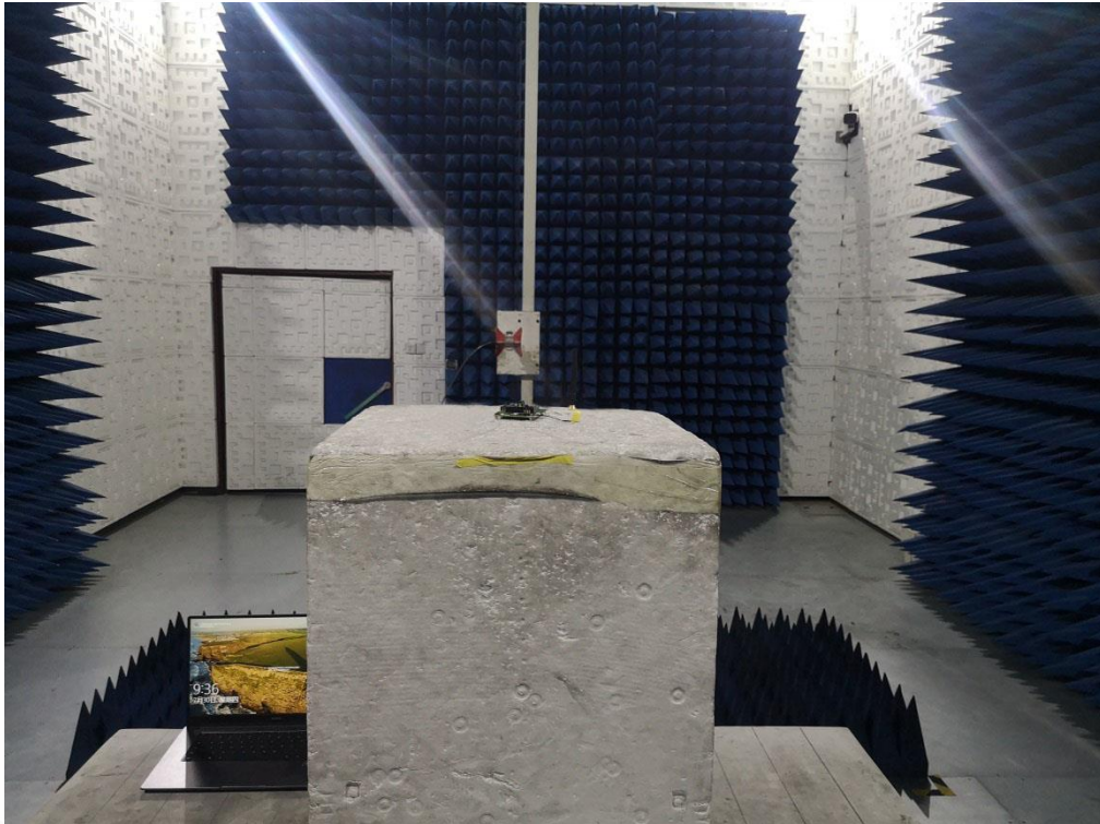
RADIATED EMISSION TEST SETUP ABOVE 1GHZ
