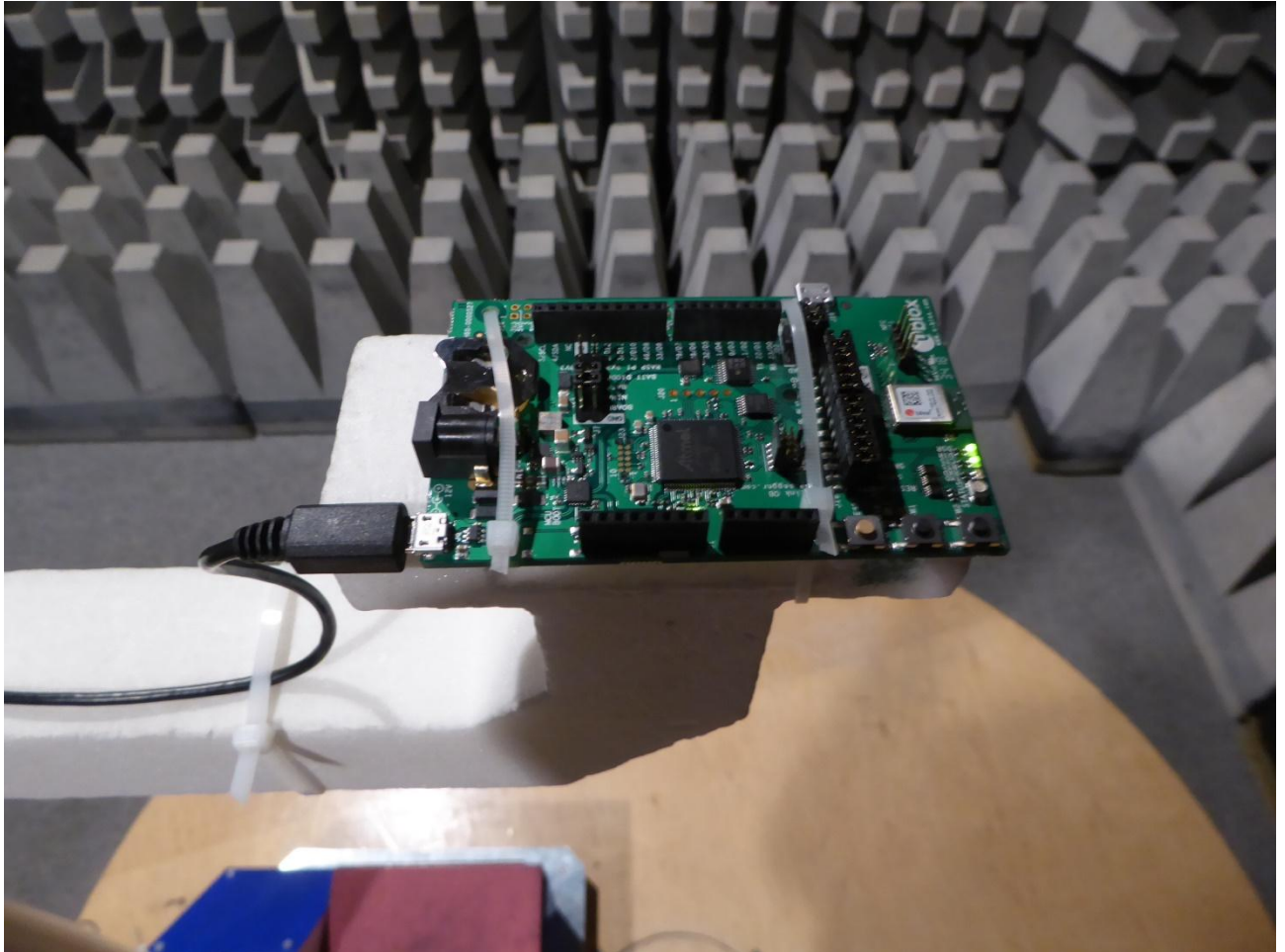
Test setup fully anechoic chamber 30 MHz – 1 GHz
