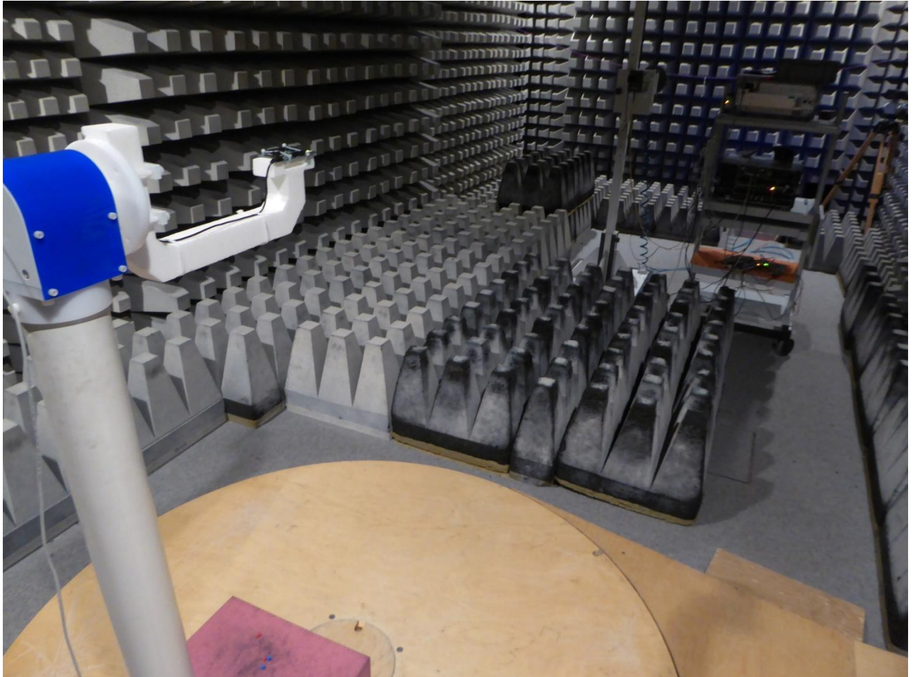
Test setup fully anechoic chamber 18 – 26.5 GHz
