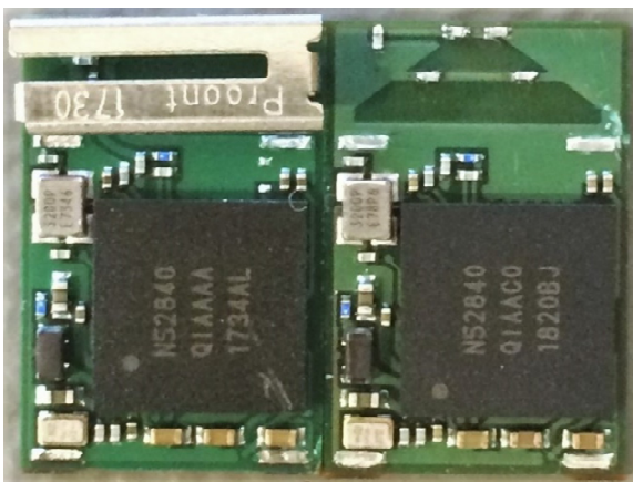
Figure 1: Antenna configuration comparison - NINA-B312 to the left, NINA-B316 to the right
