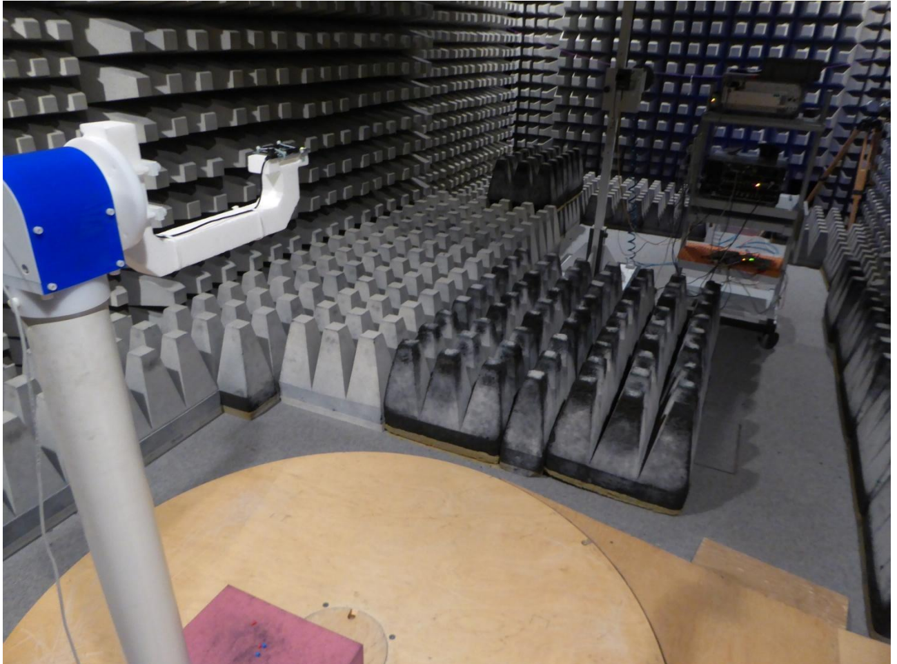
Test setup fully anechoic chamber 18 – 26.5 GHz
