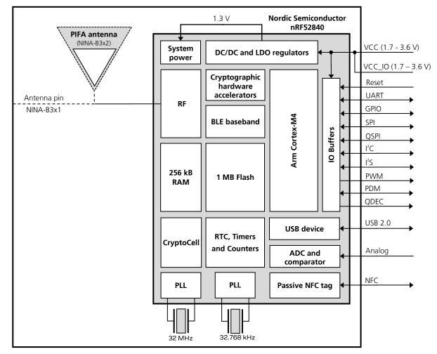
Figure 1: Block diagram of NINA-B3 series
