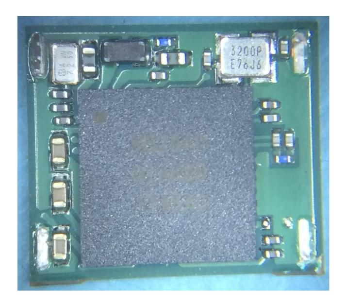
NINA-B3x1\_internal\_photo<sup>\*1</sup>: EUT NINA-B3 series without trace design – without shielding photos provided by the applicant
