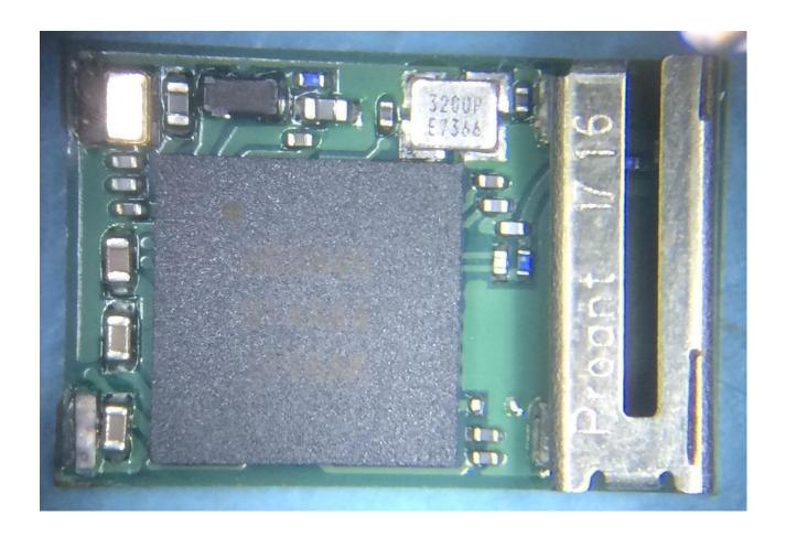
NINA-B3x1\_internal\_photo\*1: EUT NINA-B3 series with integral u-blox LILY Antenna – without shielding
