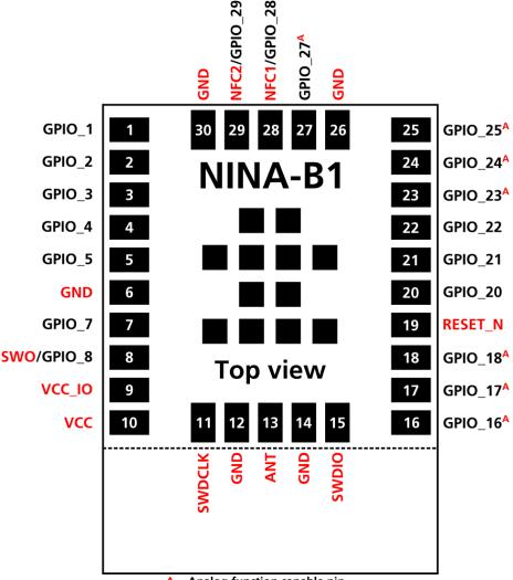
A = Analog function capable pin
