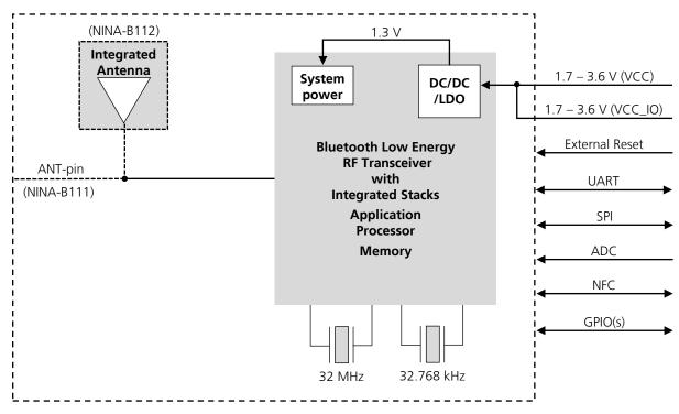
Figure 1: Block diagram of NINA-B1
