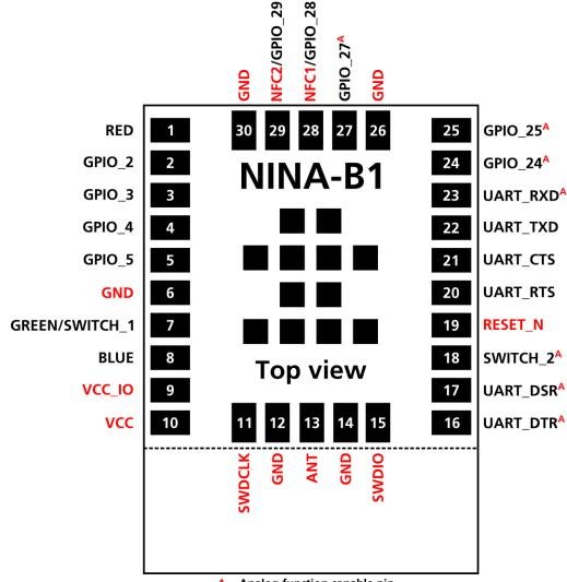
A = Analog function capable pin
