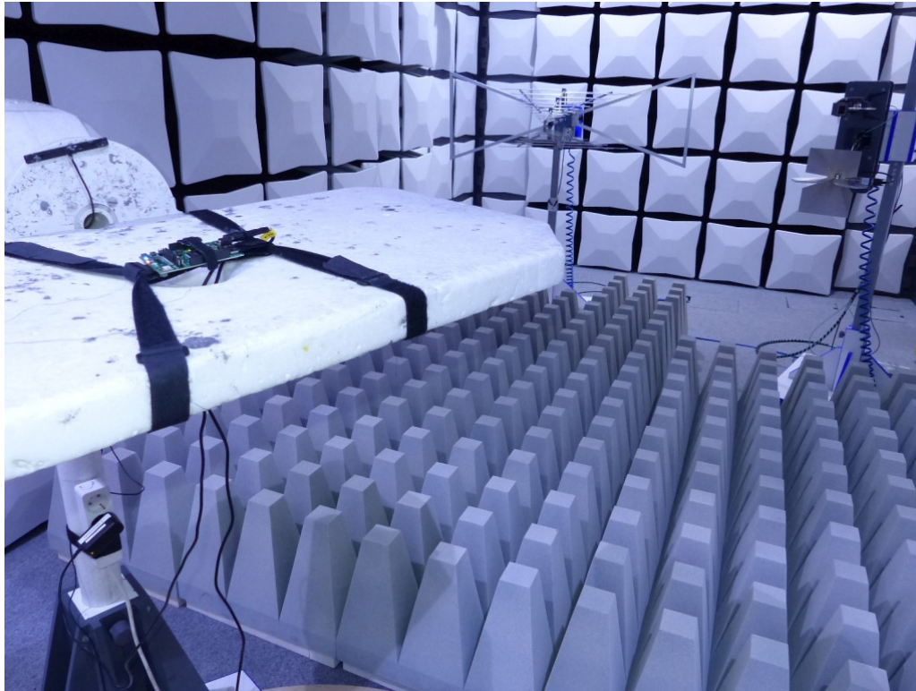
Photo 5: Test setup for radiated measurements above 1 GHz
