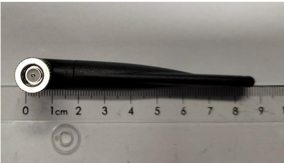
Figure 10: Antenna length _ photo to show the antenna connector.
