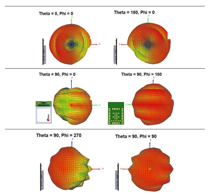
Table 3: Wi-Fi antenna characteristics at 5.50 GHz
