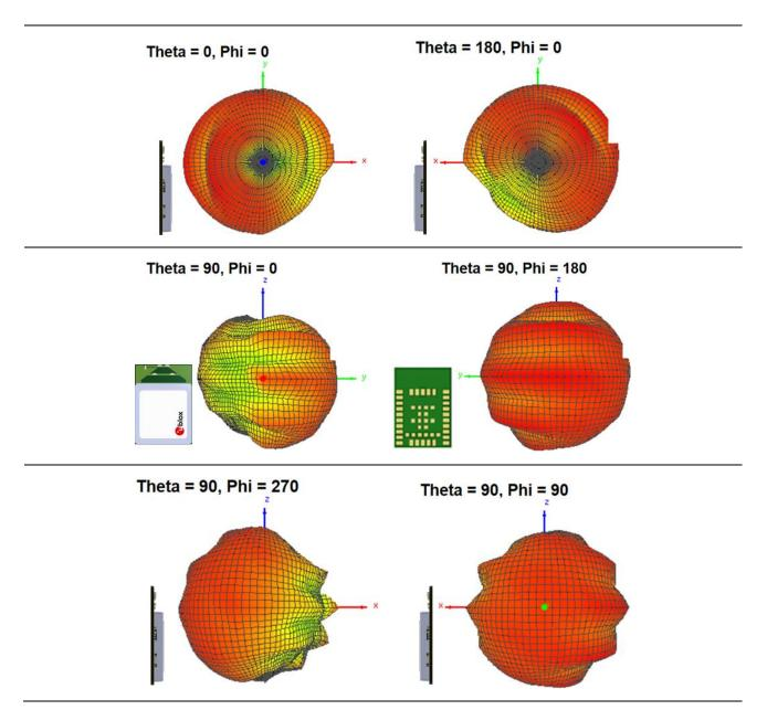
Table 3: Wi-Fi antenna characteristics at 5.50 GHz**Error! Reference source not found.** Table 2 and Table 3 show the radiation diagrams of the antenna in the middle of each frequency band, 2G and 5G respectively.
