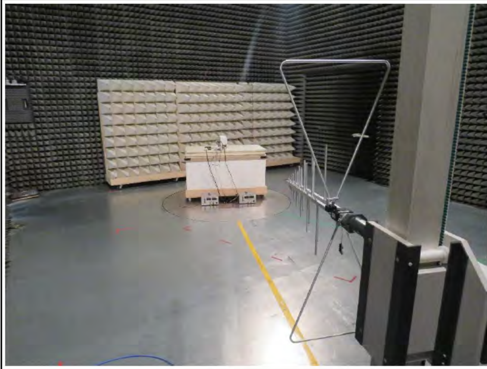
Setup for measurements below 1 GHz
