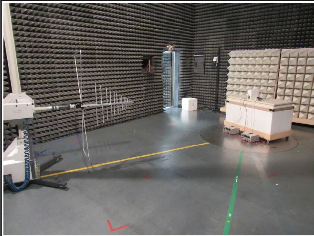
Setup for measurements below 1 GHz (2)
