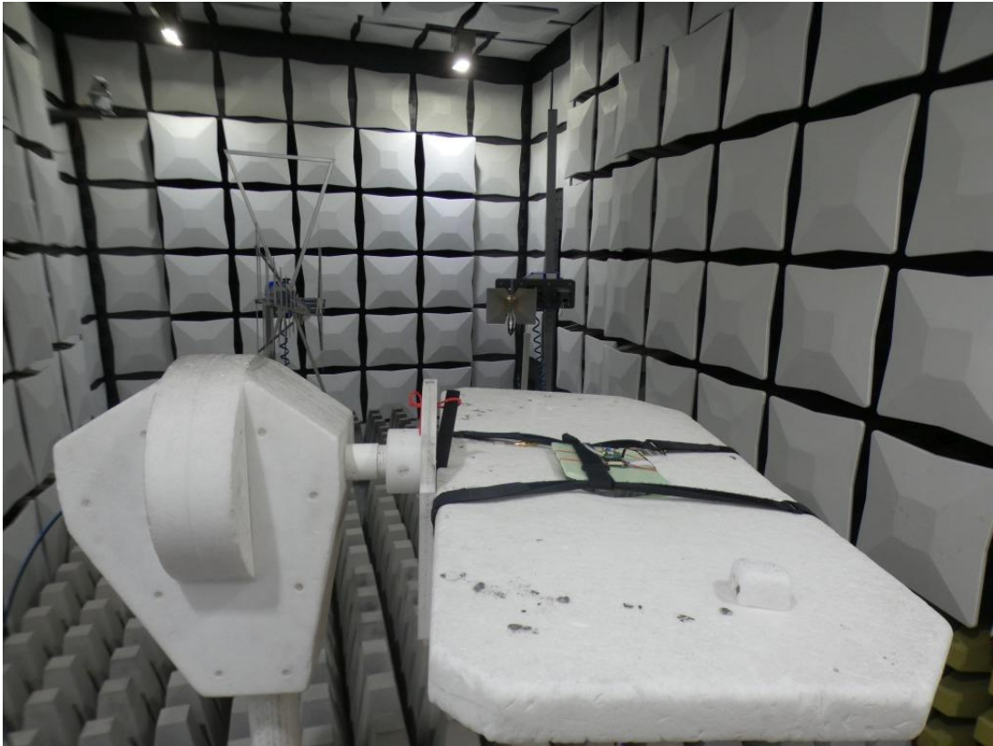
Photo 3: Test setup for radiated measurements above 26 GHz
