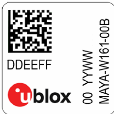
Figure 1: Label of the MAYA-W1 modules
