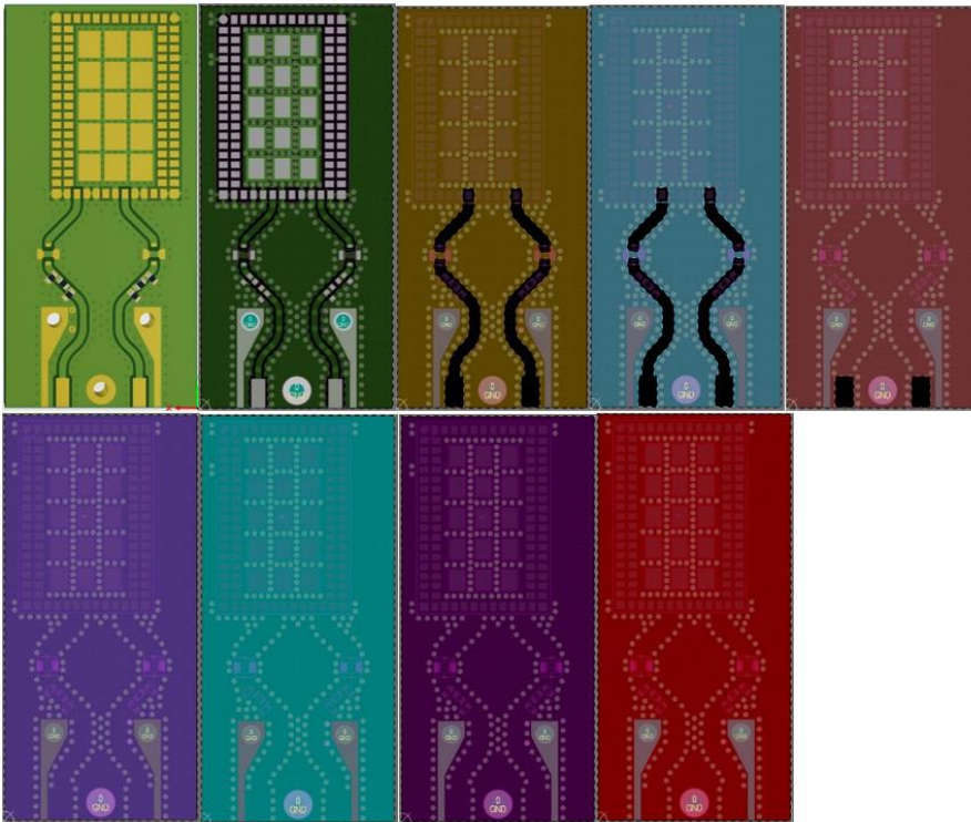
Figure 9: RF trace and ground design example
