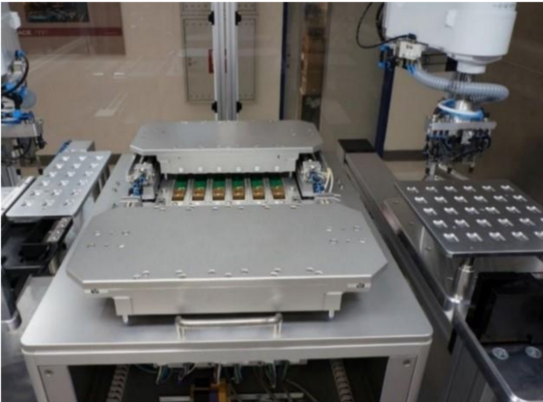
Figure 21: Automatic test equipment for module test
