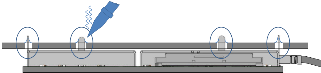
Figure 48: Shielding can soldering on baseboard by metal tabs
