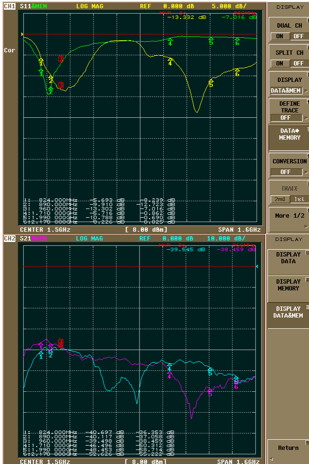
Figure 43: |S_{11}| and |S_{21}| comparison between a 900 MHz tuned half wavelength dipole and a penta-band internal antenna, if |S_{21}| like in marker 3 area are similar the target antenna performances are good
