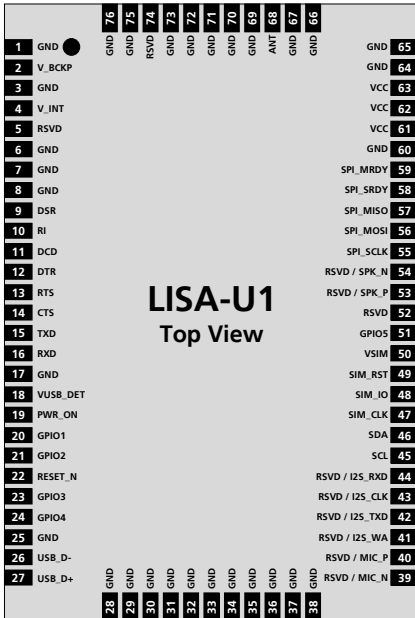
Figure 75: LISA-U1 series pin assignment
