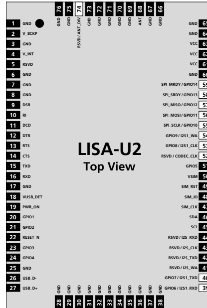
Figure 76: LISA-U2 series pin assignment (highlighted name/function changes)
