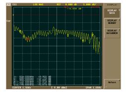
Figure 64: |S<sub>11</sub>| sample measurement of a wideband antenna
