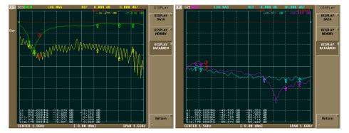
Figure 66: |S<sub>11</sub>| and |S<sub>21</sub>| comparison between a 900 MHz tuned half wavelength dipole (green/purple) and a wideband commercial antenna (yellow/cyan)
