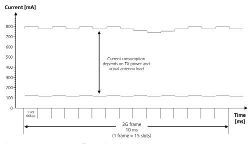
Figure 13: VCC current consumption profile versus time during a UMTS/HSPA connection
