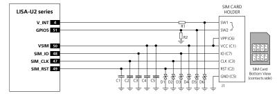
Figure 23: Application circuit for the connection to a single removable SIM card, with SIM detection implemented
