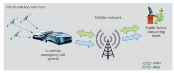
Figure 69: eCall and ERA-GLONASS automated emergency response systems diagram flow
