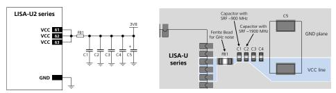
Figure 9: Suggested schematic and layout design for the VCC line; highly recommended when using an integrated antenna
