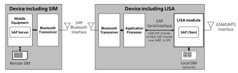
Figure 71: Remote SIM access via Bluetooth and wired connection
