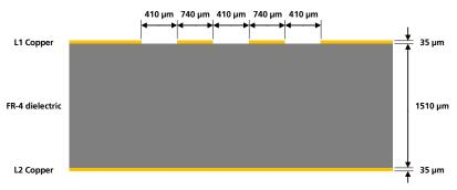
Figure 60: Example of USB line design, with Z $_{\circ}$  close to 90  $\Omega$  and Z $_{cm}$  close to 30  $\Omega$ , for the described 2-layer board layup
