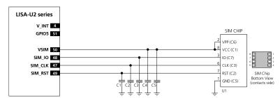
Figure 22: Application circuit for the connection to a single solderable SIM chip, with SIM detection not implemented
