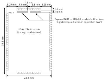
Figure 80: Signals keep-out areas on the top layer of the application board, below LISA-U2 series modules
