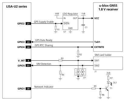
Figure 52: GPIO application circuit
