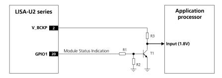
Figure 53: Module status indication application circuit
