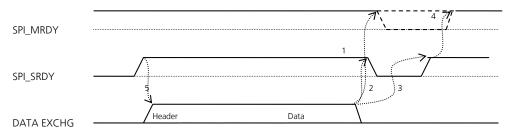
Figure 44: Data transfer terminated and then restarted by LISA-U2 module (slave)
