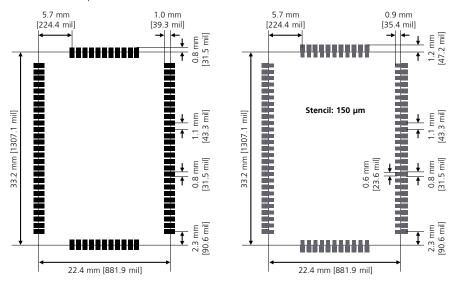
Figure 61: LISA-U2 modules suggested footprint and paste mask
