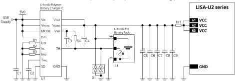
Figure 10: Li-Ion (or Li-Polymer) battery charging application circuit
