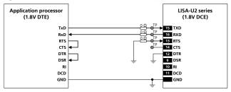
Figure 37: UART interface application circuit with partial V.24 link (3-wire) in the DTE/DCE serial communication (1.8V DTE)
