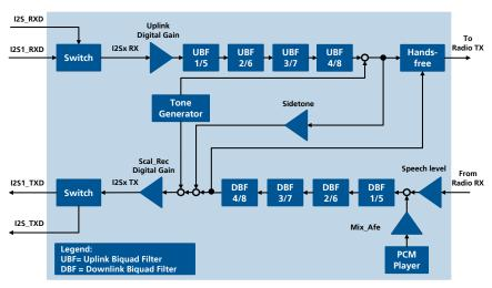
Figure 51: Audio processing system of LISA-U2 series modules
