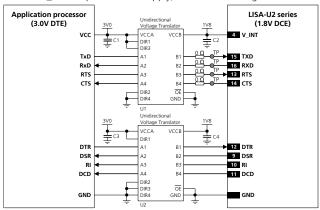
Figure 32: UART interface application circuit with complete V.24 link in DTE/DCE serial communication (3.0 V DTE)
