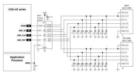
Figure 24: Application circuit for the connection to two removable SIM cards, with SIM detection implemented
