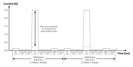
Figure 11: VCC current consumption profile versus time during a GSM call (1 TX slot, 1 RX slot)
