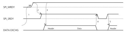
Figure 43: Data transfer initiated by application processor (master) with a sleeping LISA-U2 module (slave)
