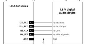
Figure 49: I<sup>2</sup>S interface application circuit with a generic digital audio device
