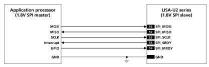
Figure 45: IPC / SPI Interface application circuit connecting LISA-U2 series 1.8V SPI slave to a 1.8V SPI master
