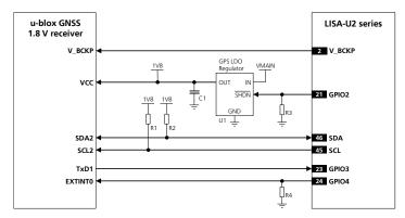
Figure 47: DDC Application circuit for u-blox 1.8 V GNSS receiver
