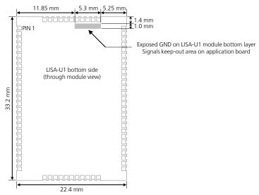
Figure 79: Signals keep-out area on the top layer of the application board, below LISA-U1 series modules
