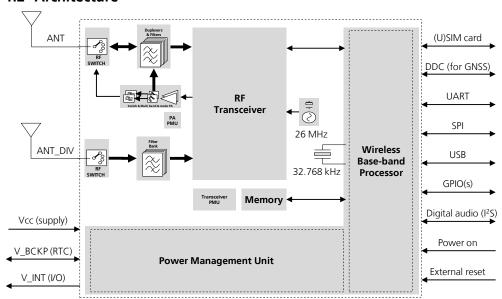
Figure 1: LISA-U2 series block diagram (for available options see Table 2)
