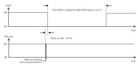
Figure 29: Wake-up via data reception without further communication
