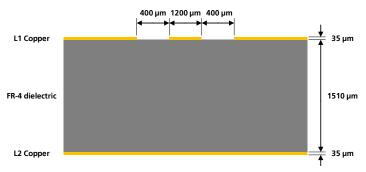
Figure 58: Example of 50  $\Omega$  coplanar waveguide transmission line design for the described 2-layer board layup
