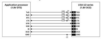
Figure 31: UART interface application circuit with complete V.24 link in DTE/DCE serial communication (1.8V DTE)
