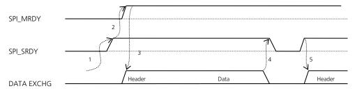
Figure 42: Data transfer initiated by LISA-U2 module (slave), with a sleeping application processor (master)
