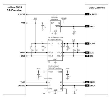
Figure 48: DDC Application circuit for u-blox 3.0 V GNSS received
