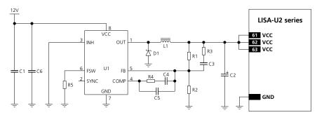
Figure 7: Suggested low cost solution for the VCC voltage supply application circuit using step-down regulator
