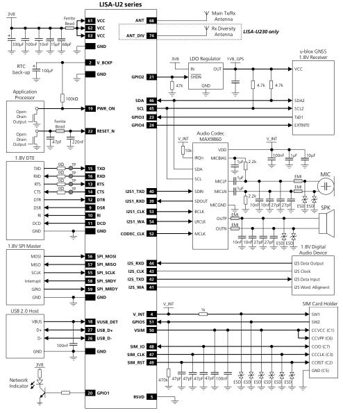
Figure 54: Example of schematic diagram to integrate LISA-U2 series modules in an application board, using all the interfaces
