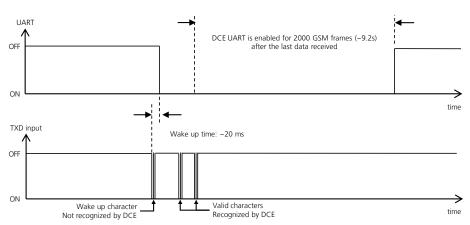
Figure 30: Wake-up via data reception with further communication
