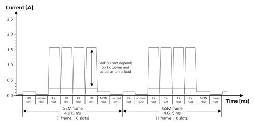
Figure 12: VCC current consumption profile versus time during a GPRS/EDGE connection (4TX slots, 1 RX slot)
