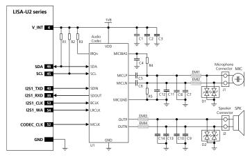
Figure 50: I'S interface application circuit with an external audio codec to provide voice capability
