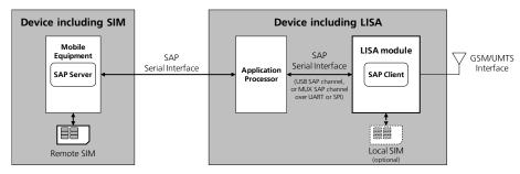
Figure 70: Remote SIM access via completely wired connection
