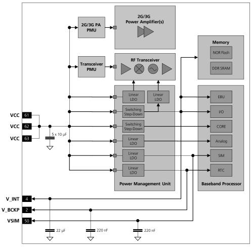
Figure 3: LISA-U2 series power management simplified block diagram
