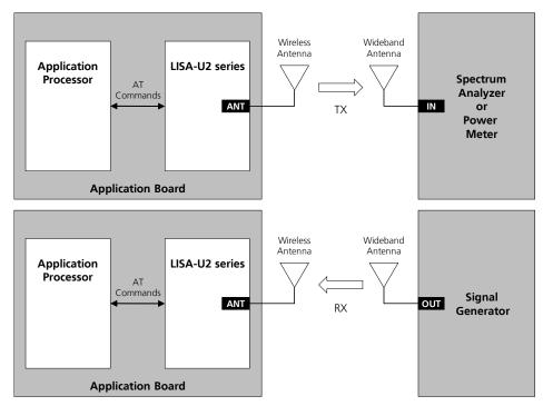
Figure 76: Setup with spectrum analyzer and signal generator for radiated measurement
