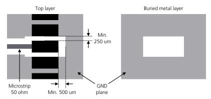
Figure 56: GND keep-out area on top layer around ANT and ANT\_DIV pads and on buried layer below ANT and ANT\_DIV pads
