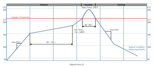
Figure 74: Recommended soldering profile
