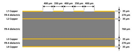
Figure 59: Example of USB line design, with  $Z_{\circ}$  close to 90  $\Omega$  and  $Z_{cM}$  close to 30  $\Omega$ , for the described 4-layer board layup
