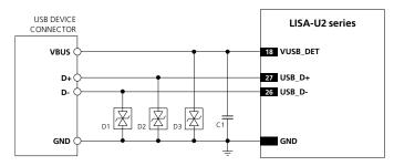
Figure 40: USB Interface application circuit
