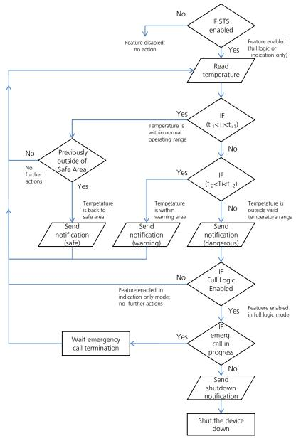
Figure 73: Smart Temperature Supervisor (STS) flow diagram
