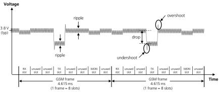
Figure 4: Description of the VCC voltage profile versus time during a GSM call
