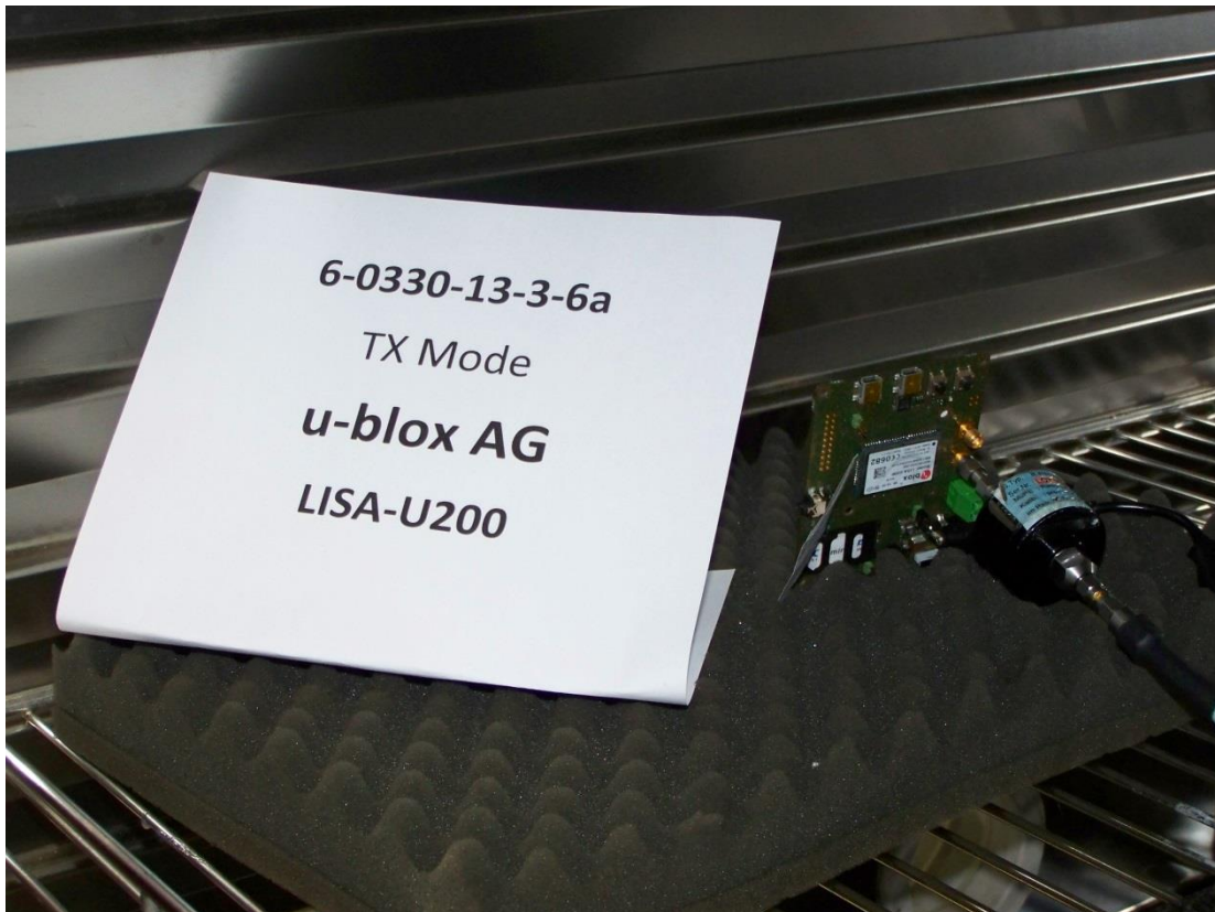
Conducted RF-measurements at the Radio laboratory 1 (in the climatic chamber), test setup 2
