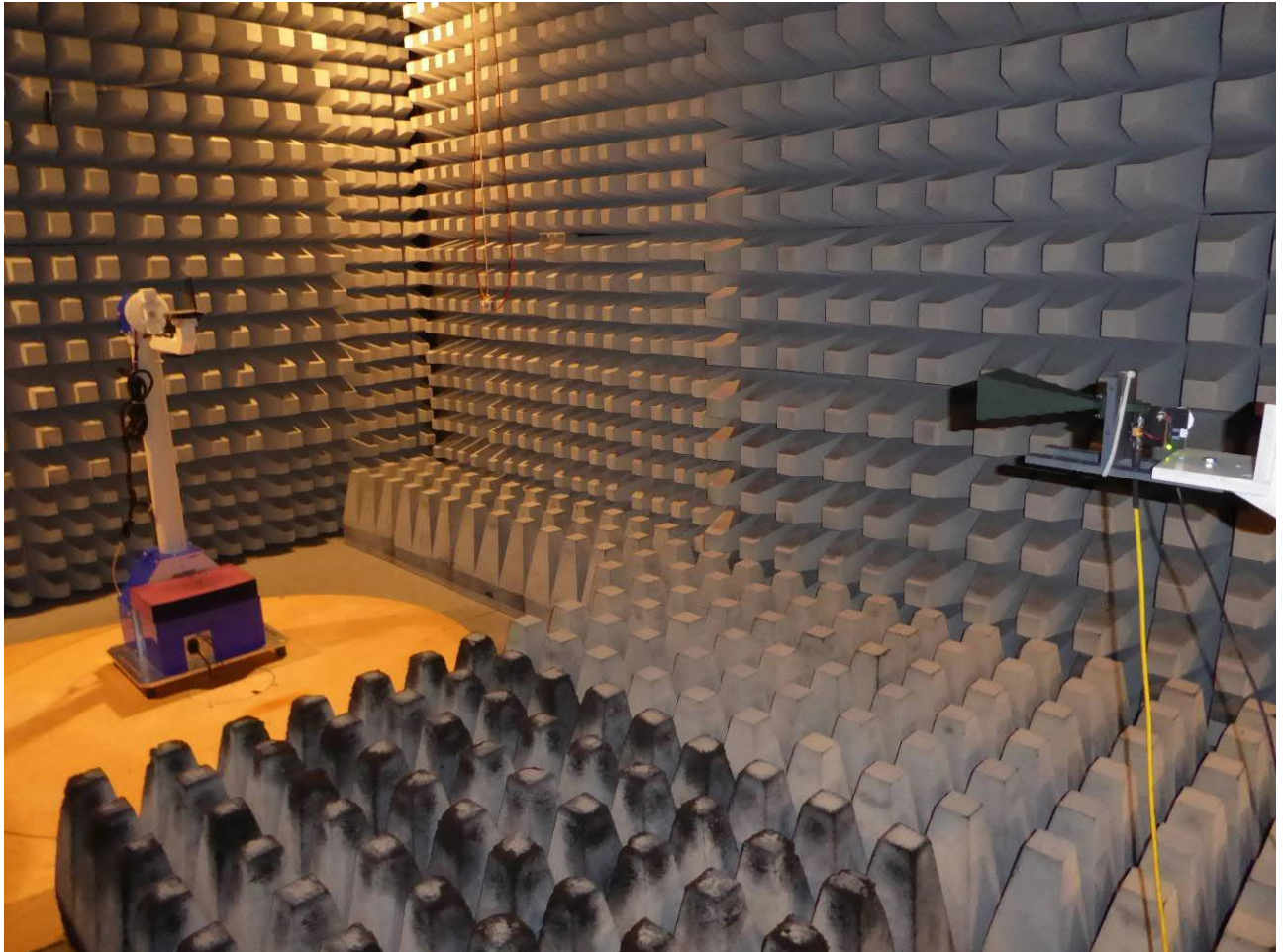
Test setup – radiated test in anechoic chamber (M20)
