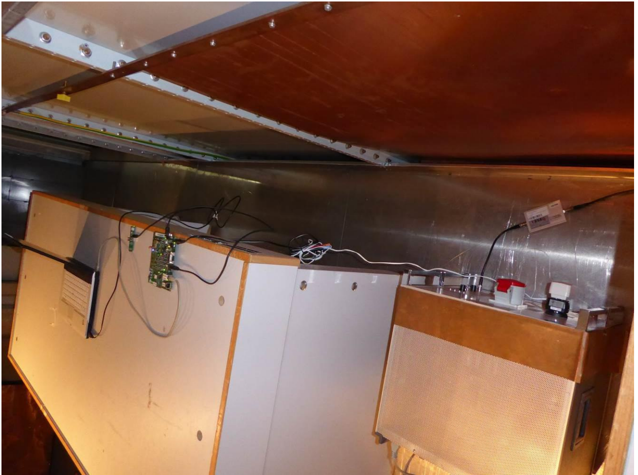
160307_25: Test setup – conducted emissions on power supply lines
