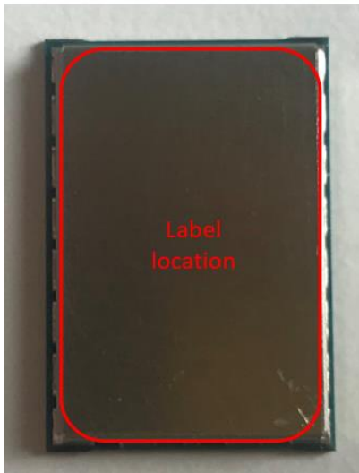
Figure 3: Label location of the JODY-W5 modules
