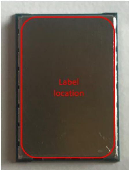
Figure 3: Label location of the JODY-W3 modules
