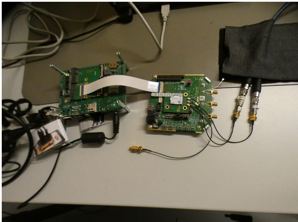
Photo 2: Test setup for conducted DFS tests, EUT detail
