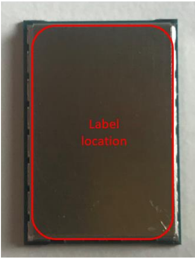
Figure 9: Label location of the JODY-W3 modules
