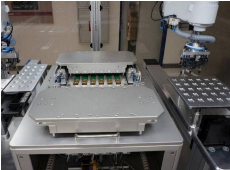
Figure 17: Automatic test equipment for module test
