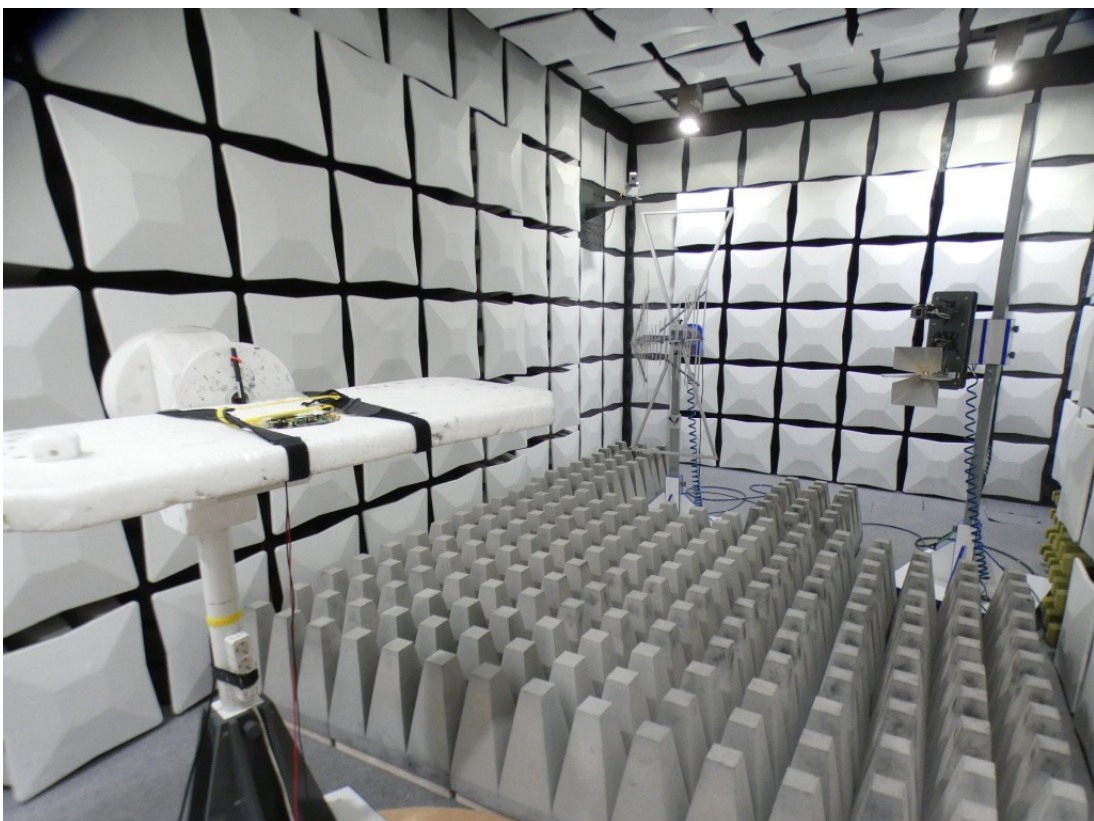
Photo 4: Test setup for radiated measurements above 1 GHz
