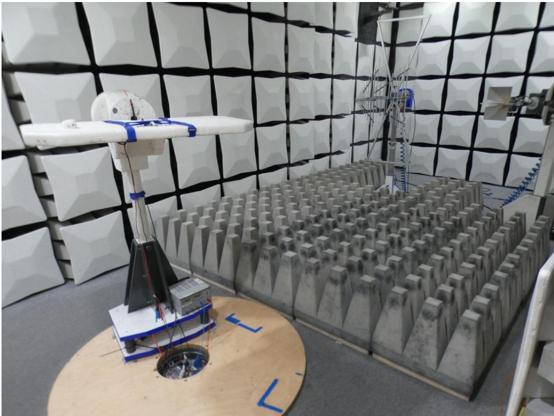
Photo 3: Test setup for radiated measurements above 1 GHz
