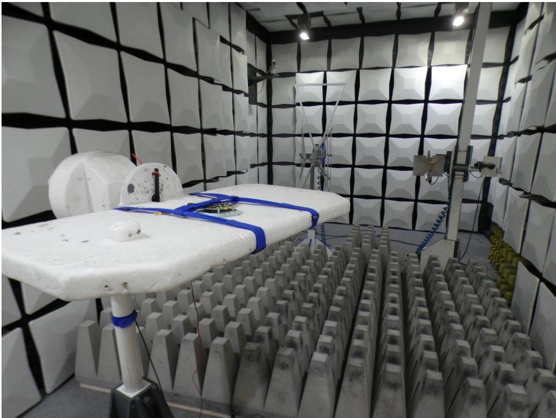
Photo 3: Test setup for radiated measurements above 1 GHz
