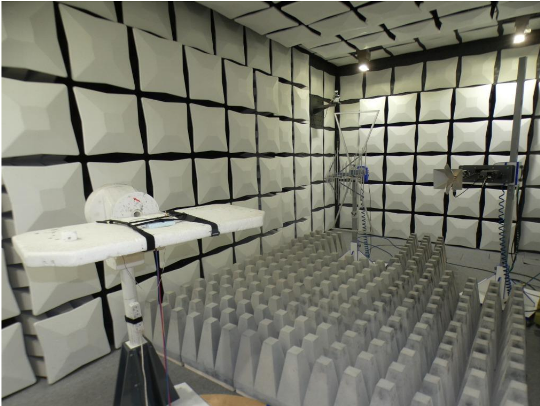
Photo 3: Test setup for radiated measurements above 26 GHz
