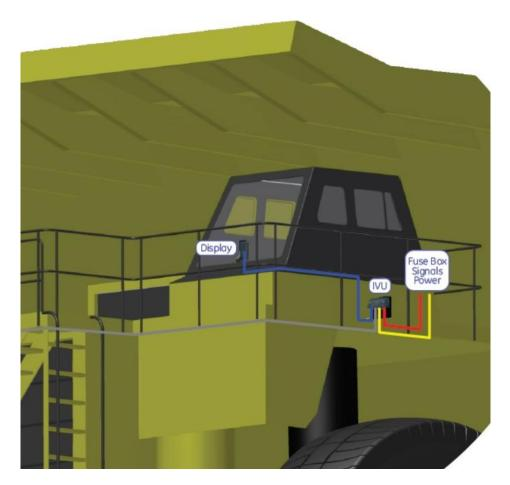
Note: IVU preferably mounted inside the Operator's cabin or the electrical compartment
